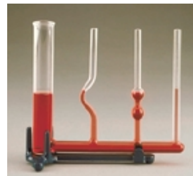
Figure 4.31 Pascal's vases show that a container's shape has no effect on pressure.
