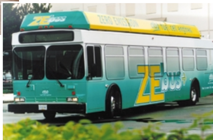
Figure 4.69C This bus is fuelled by a hydrogen fuel cell.
