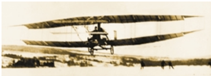
Figure 4.62A The Silver Dart was the first powered airplane flown in Canada. It was designed in 1909 by Canadian J.A.D. McCurdy, a member of Alexander Graham Bell's Aerial Experiment Association. To launch the plane, a horse-drawn sleigh pulled it over the ice of Baddeck Bay in Cape Breton. The plane rose after being pulled about 30 m, and flew at an elevation of 3 to 9 m and a speed of 65 km/h for 0.8 km.
