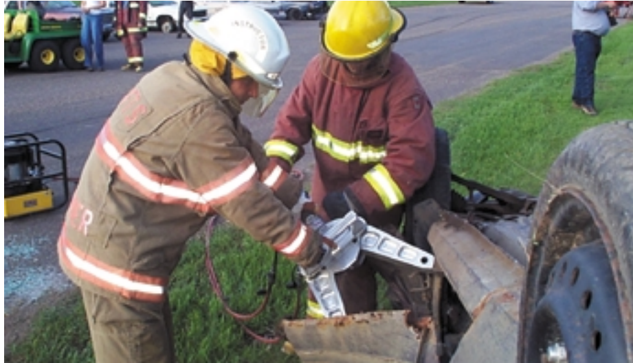
Randy shows Richelle how to use a heavy hydraulic spreader to force open a car door.
