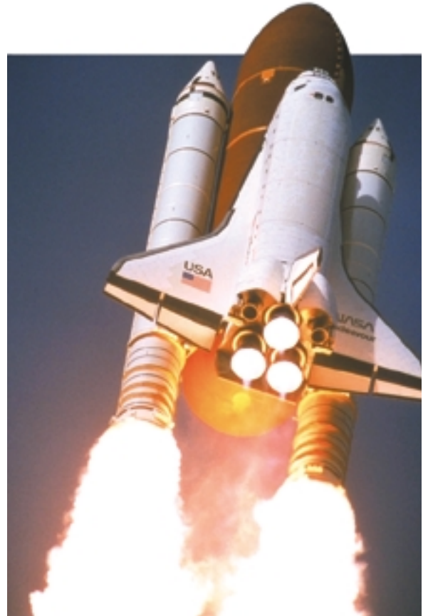
Figure 4.62B The Space Shuttle is a spacecraft that consists of a winged orbiter and booster rockets that propel the craft into space. About two minutes after lift off, the boosters use up their fuel, separate from the spacecraft and re-enter the atmosphere, where they are retrieved. After completion of the space mission, the orbiter reduces its speed, descends through the atmosphere, and lands like an airplane.
