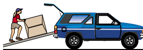
Figure 4.7B Olivia used an inclined plane to help her load the box of camping gear into the truck. The inclined plane decreased the effort force Olivia needed by increasing the distance through which her effort force was applied.
