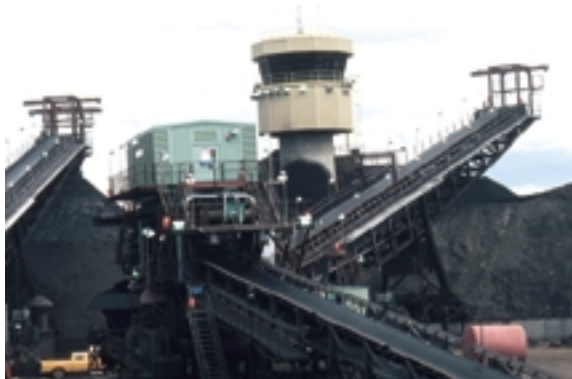
Figure 4.20 This enormous conveyor belt is used at Syncrude Oil Sands in Fort McMurray, Alberta. The belt acts like a chain. Can you see the sprockets?
