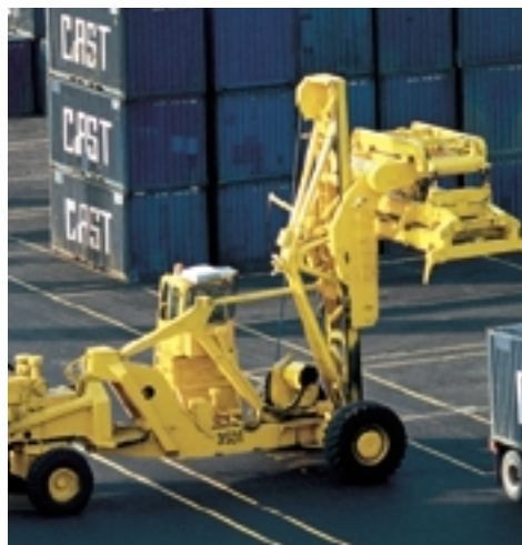
Figure 4.32B Powered hydraulically, this forklift can move very large containers.
