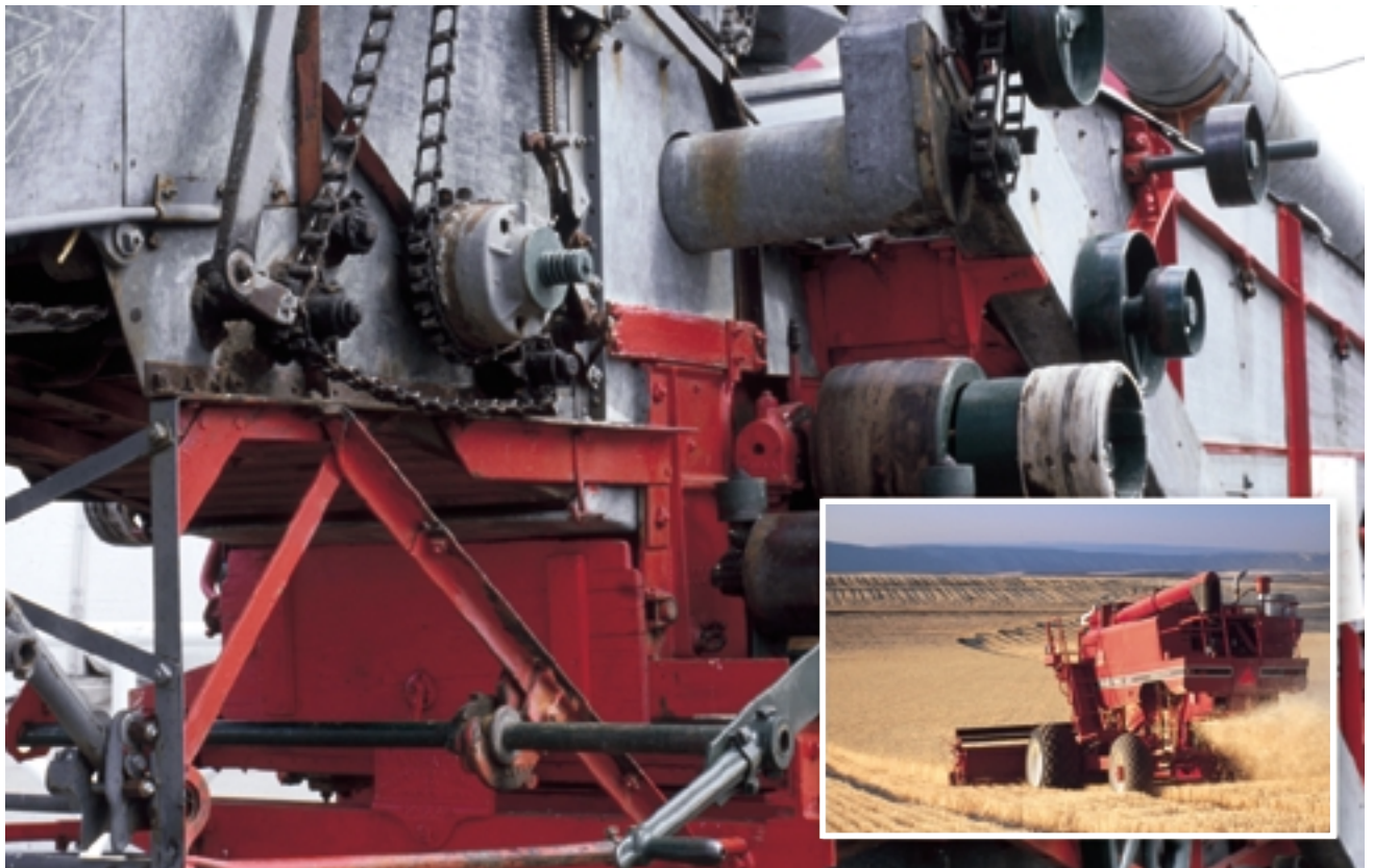
Figure 4.16 This combine features sprockets and belts, as well as a gear train.
