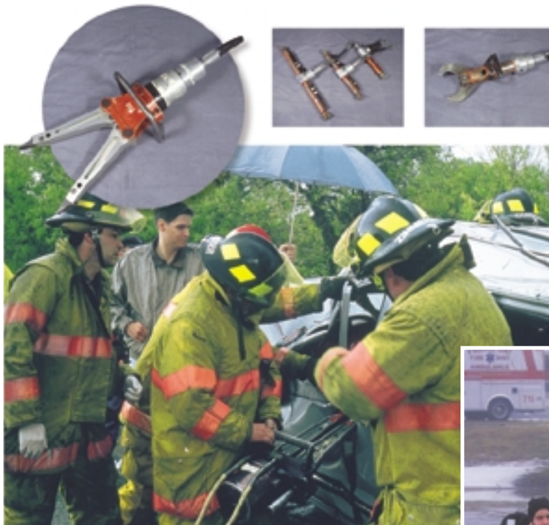
Figure 4.35 Firefighters are using the hydraulically powered Jaws of Life to rescue an accident victim from a crushed car. Above the photo are three types of tools used in the Jaws of Life (from left to right): spreaders, rams, and cutters.
