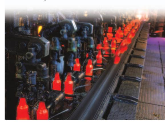
Figure 1.7 Glass bottles being formed
