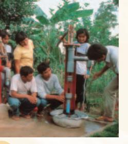
The PVC water pump is a good example of the importance of understanding a concept so that you can apply that understanding to different situations. In this case, the inventors knew about the properties of fluids and how a water pump operates. They applied this knowledge to develop a better pump that would work reliably for long hours and be easy to fix. In this unit, you will learn about the properties of fluids and see how they can be used to solve a variety of practical problems.
