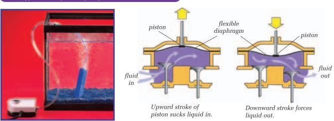
Figure 4.4 Diaphragm pumps are used for both liquids and gases, such as the air pumped into this aquarium.
