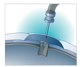
**Figure 4.9** This type of valve allows you to inflate a ball, but also keeps air from leaking out. To open the valve, you insert a hollow pin. You inflate the ball by pumping air through the pin. You deflate the ball by allowing air to escape through the pin.
