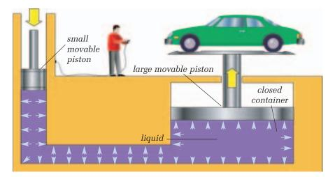
**Figure 3.20** A car lift or hoist. The arrows in the liquid indicate the pressure transmitted throughout the system. Hoists are used in repair garages so that mechanics can work under cars more easily.
