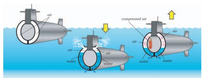
**Figure 4.14a) On the Surface**. When the submarine is on the surface, its ballast tanks are full of air. The average density of the submarine is less dense than the density of the water, and it floats. Figure 4.14b) Diving. To dive, the
