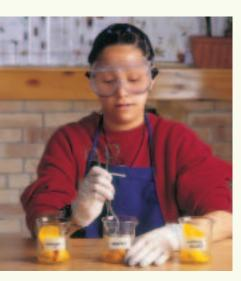
**Figure 4.2** Step 4. Swirl the fabric around in each solution using the forceps.
