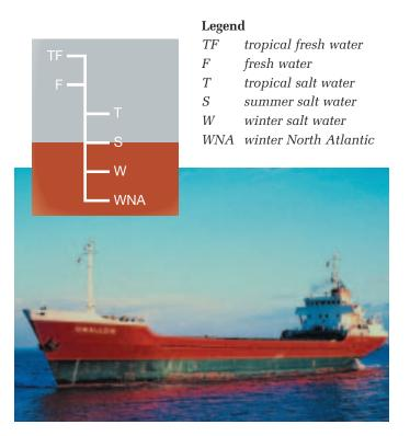
**Figure 3.11** The Plimsoll line indicates how heavily loaded a ship can be in different densities of water.
