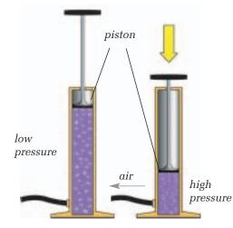
**Figure 4.6** When force is applied to the air in the cylinder, the pressure increases.
