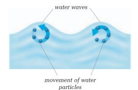
**Figure 2.4** A wave moves along the surface of the water, but the water itself moves only in a tiny circle in one place.
