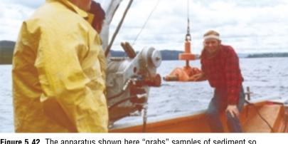
**Figure 5.42** The apparatus shown here "grabs" samples of sediment so scientists can analyze them in a laboratory.
