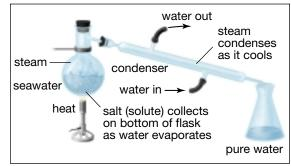
Figure 5.96B The process of distillation
