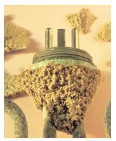
**Figure 5.85** This electric kettle element shows deposits of salts left by water evaporation.
