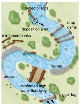
erosion, reinforced rock baskets, called rip-rap, may be necessary. To help deepen the river channel, "digger logs" are sometimes installed to force water down.
